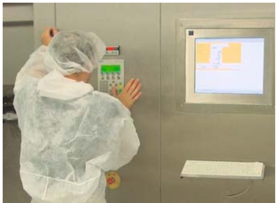
Reinraum-PC in Edelstahlwand. Clean-room PC in stainless steel wall panel.
