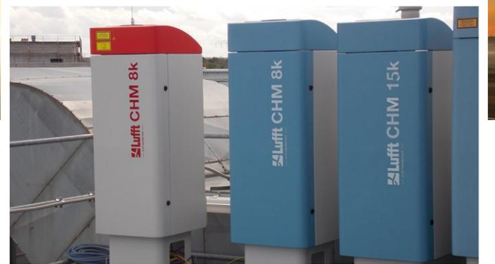
One important use of the ceilometer is to determine cloud ceilings at airports. CHM 8k can identify up to 9 cloud layers and is very sensitive even at ground level.
