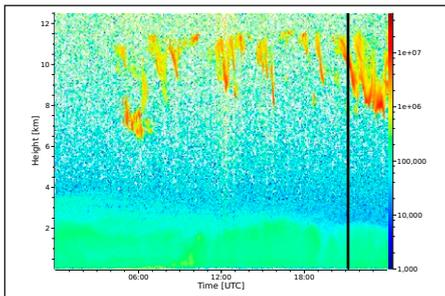
The graphical view of backscatter activity shows a cirrus cloud structure over the course of the day between 6 and 12 km and an aerosol layer structure up to 2 km altitude. The related height profile (black line at 21:00 UTC) is shown at the right side of the diagram.
