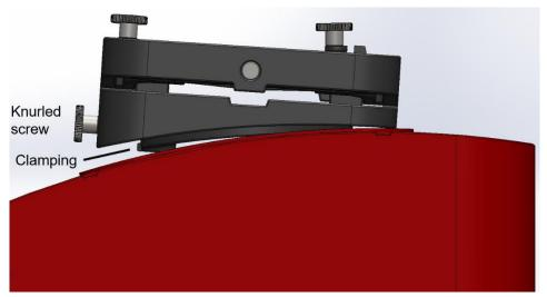
Figure 7 Fixing the angle adapter on the hood.
