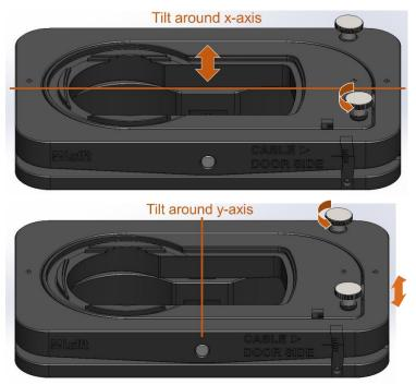
Figure 15 Alignment of the angle of both axis of the angle adapter.
