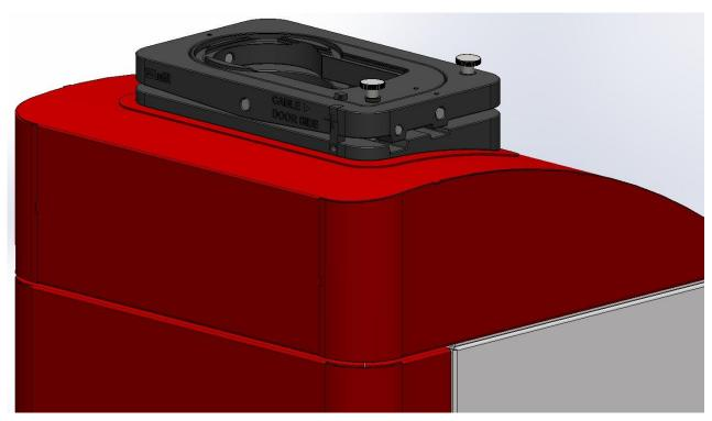
Figure 5 Alignment of the angle adapter to the ceilometer.
