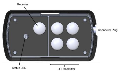
Figure 2 Components of the Cloud Height Simulator.
