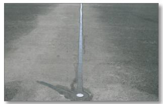
92% of all landing accidents are caused by slippery runway conditions (source: The Boeing Company). To avoid this, runway condition sensors from Lufft inform on several surface status such as temperature, water film height, ice percentage and friction.
