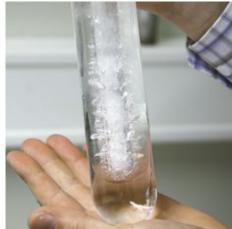
The triple point of water (balance of all 3 physical states solid, liquid and gas) is used to represent the International Temperature Scale and for the highest precision of temperature measurements in the milli-Kelvin range.
