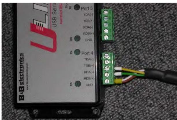
Figure 14 RS485 connection to transducer.
