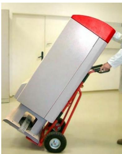
Figure 9 Transport with hand truck.
