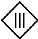
Figure 1 Symbol marking the protection class III (SELV).
