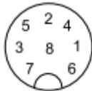
Figure 4 Pin assignment of the connector plug
