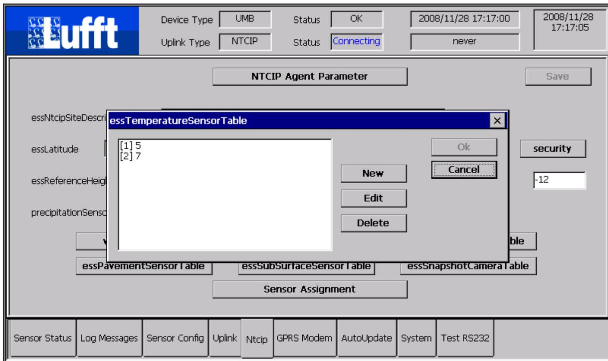
The meta data for each temperature sensor (height, location information etc.) and thereby the number of sensors in the corresponding table is configured here.
