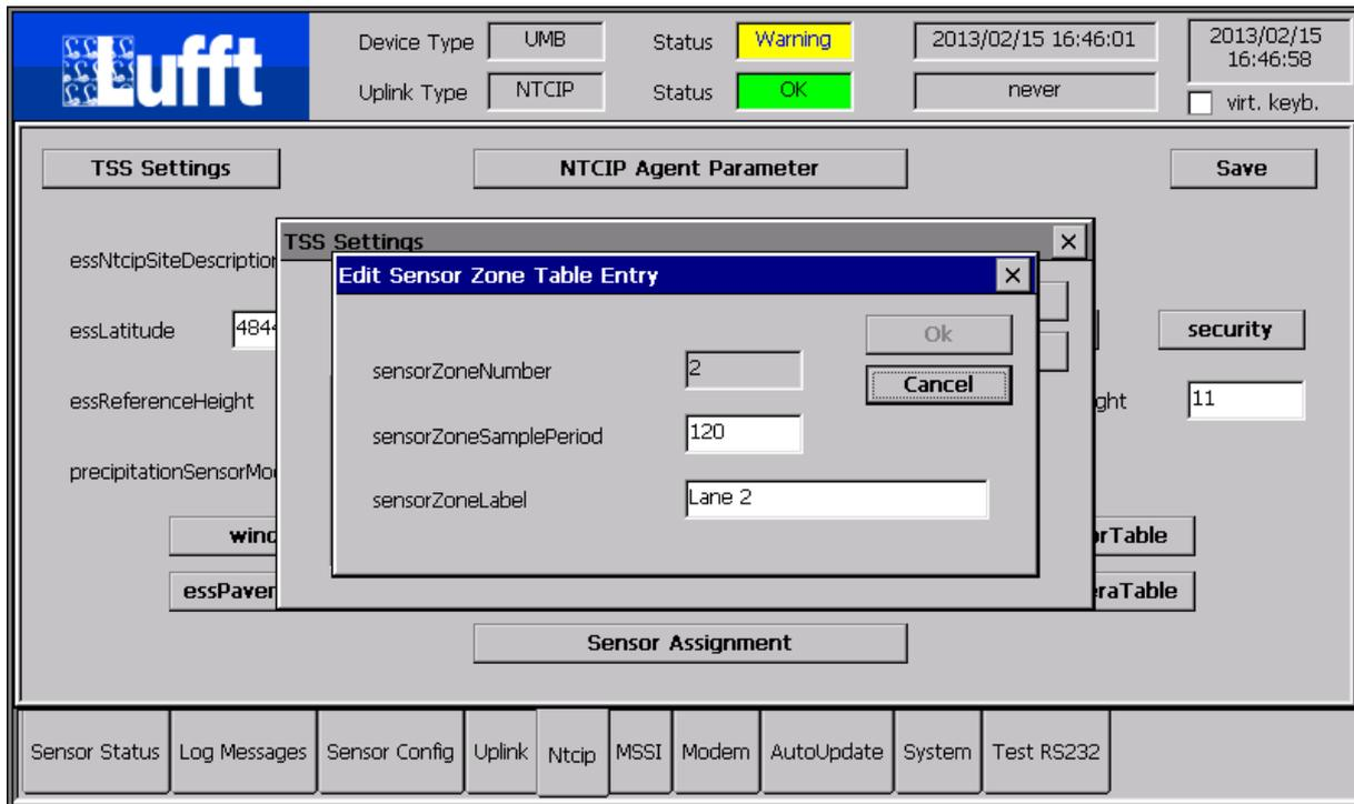
For every zone/lane, the “sensorZoneSamplePeriod” – which is the time interval used to report the data under “tss.tssDataCollection” in the “dataCollectionTable” and “dataBufferTable” – and a label for the zone/lane can be configured.
