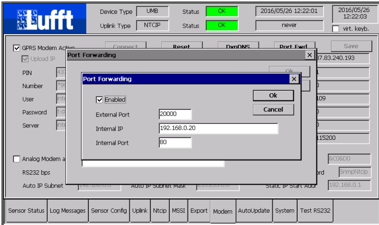
Besides the external port (i.e. the TCP port that will be available on the IP address of the GPRS modem), the internal IP address and port are configured to which this port should be redirected.
