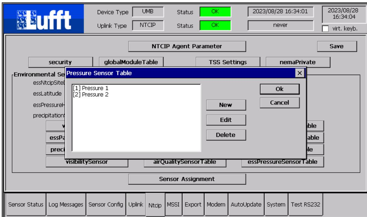
The meta data for each pressure sensor (location information etc.) and thereby the number of sensors in the corresponding table is configured here.
