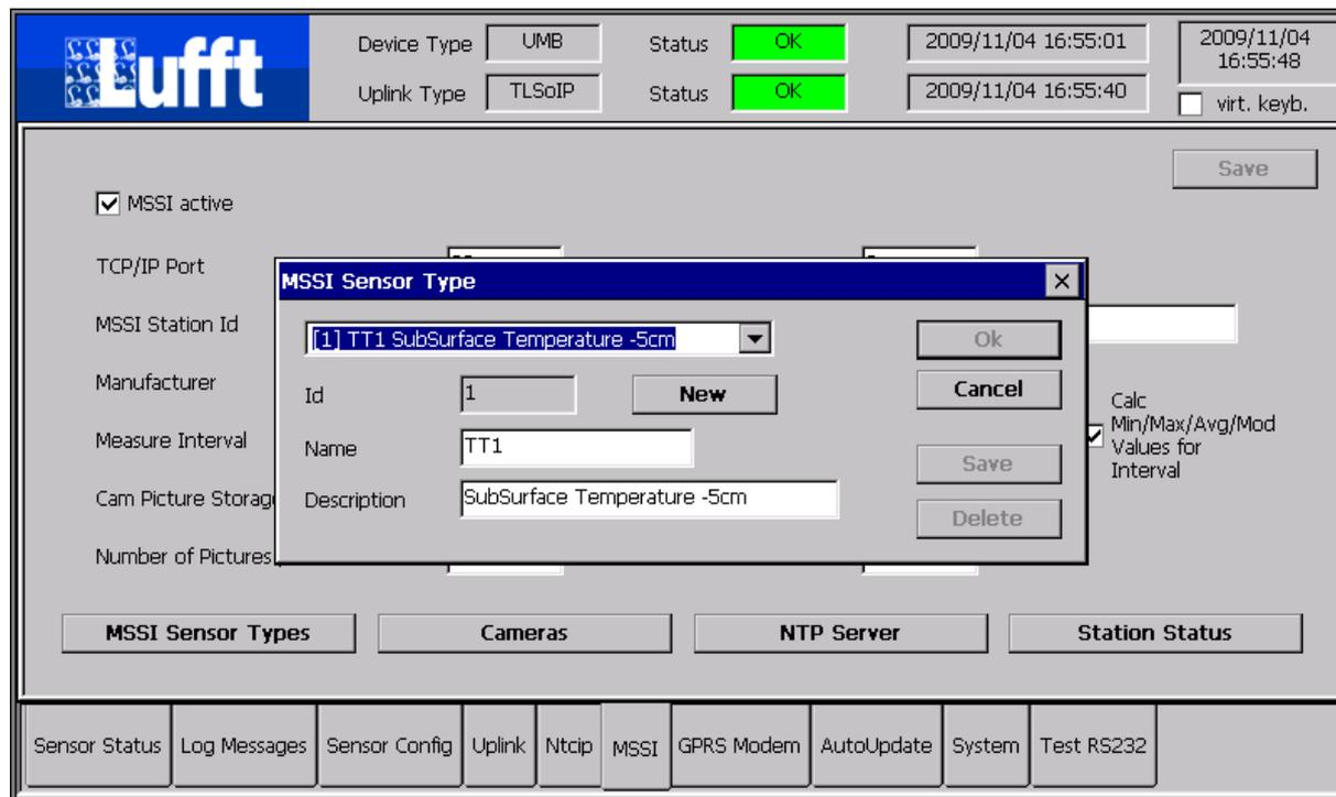
The pre-defined and user-defined types can be configured in the “MSSI Sensor Type” dialog.
