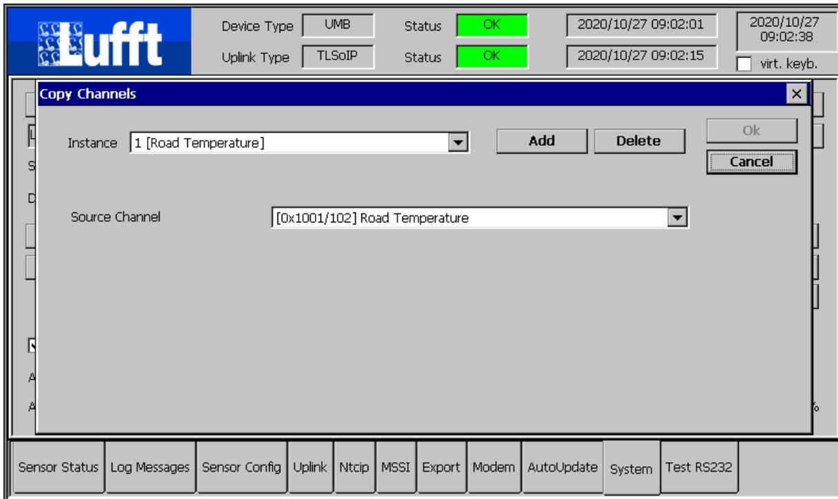
Here, copies of UMB sensor channels can be configured, e.g. if the same source channel is needed to be processed with different value mapping/scaling results.
