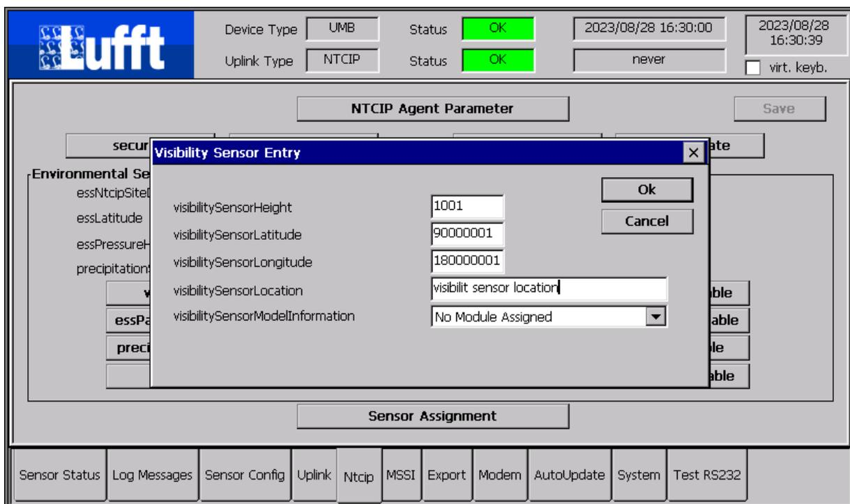
The meta data for the visibility sensor (location information etc.) is configured here.
