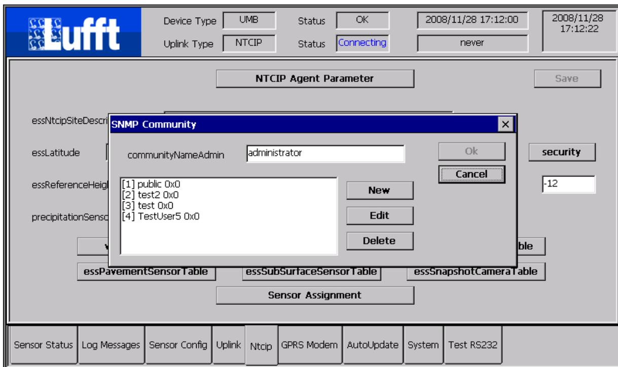
Here you can configure the entries in the SNMP security table that control the access to the SNMP protocol stack. Note: Changes cause a system reboot (after saving the changes).
