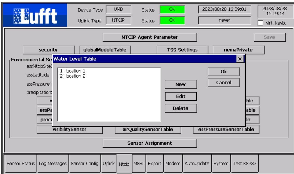
The meta data for each water level sensor (location information etc.) and thereby the number of sensors in the corresponding table is configured here.
