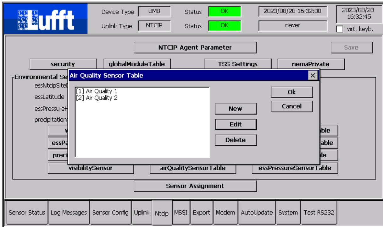
The meta data for each air quality sensor (location information etc.) and thereby the number of sensors in the corresponding table is configured here.
