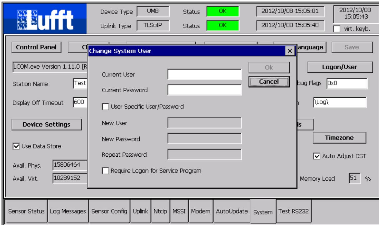
Here the system user and password can be configured. This user and password are used for
