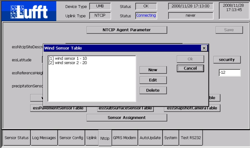
The meta data for each wind sensor (location information etc.) and thereby the number of sensors in the corresponding table is configured here.
