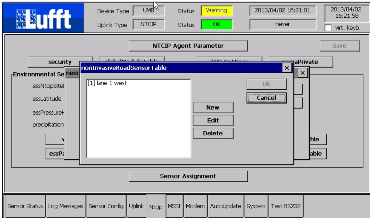
The nonInvasiveRoadSensorTable is used to configure the number of NIR Sensors.
