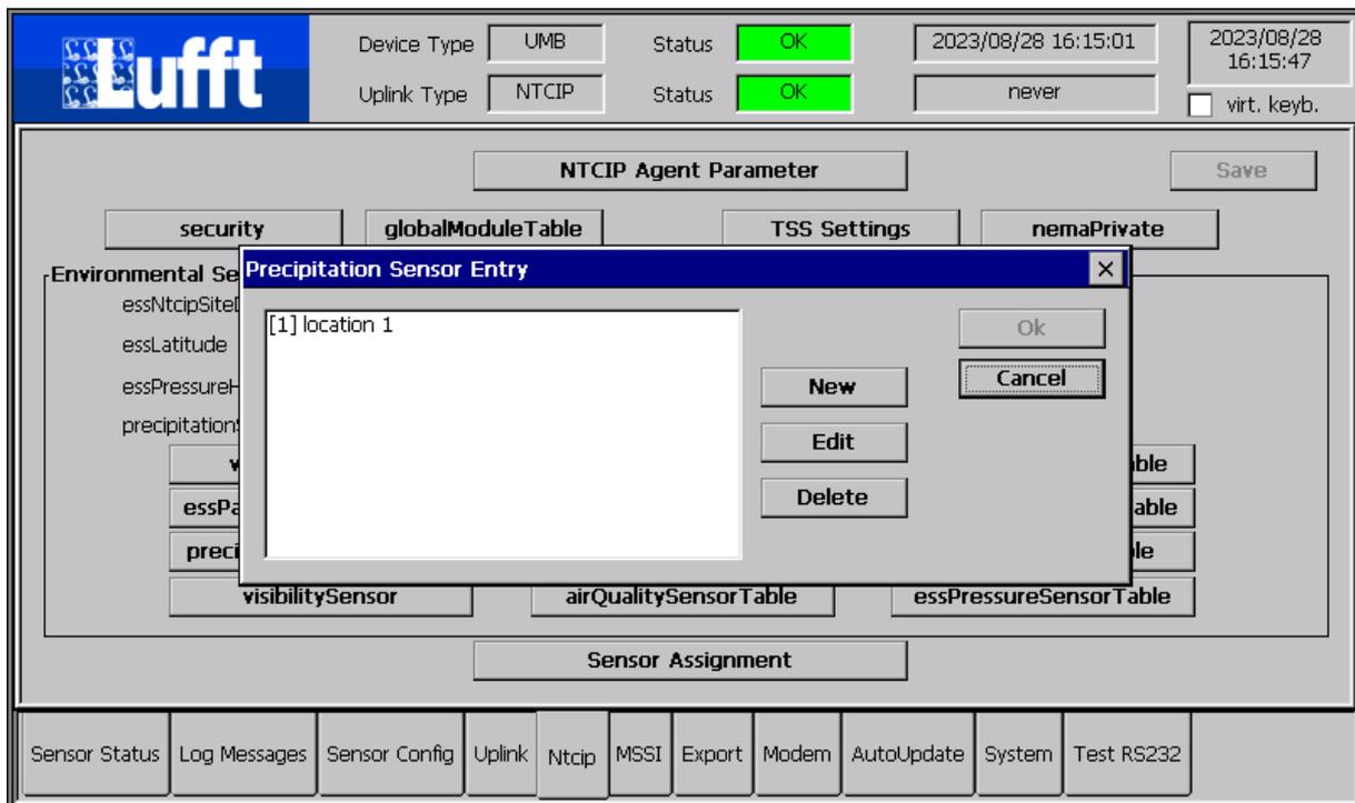
The meta data for each precipitation sensor (location information etc.) and thereby the number of sensors in the corresponding table is configured here.
