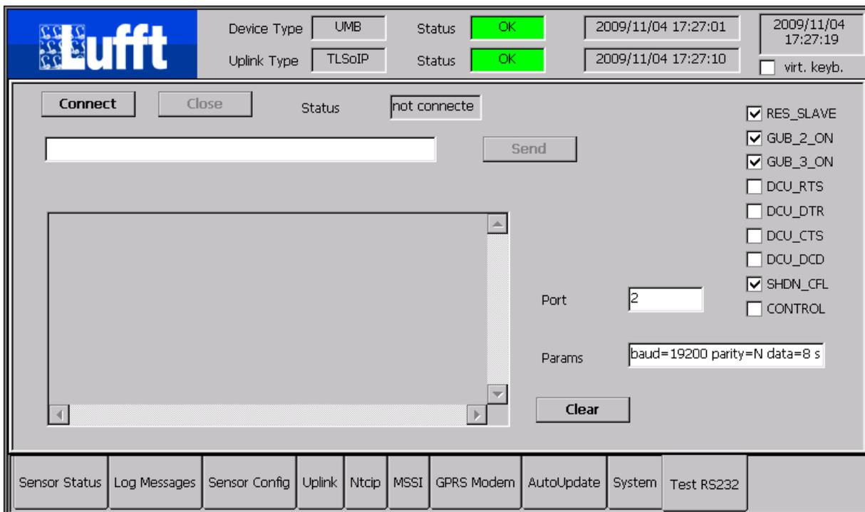
A simple test application for RS232 interfaces.
