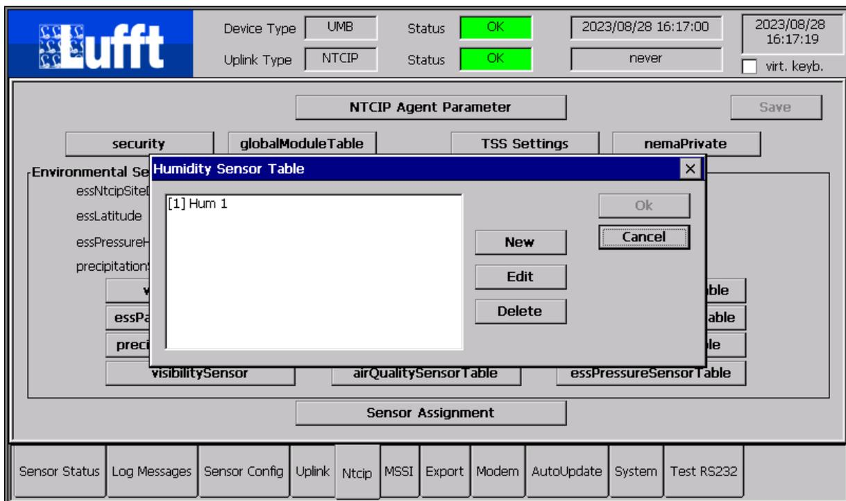
The meta data for each humidity sensor (location information etc.) and thereby the number of sensors in the corresponding table is configured here.
