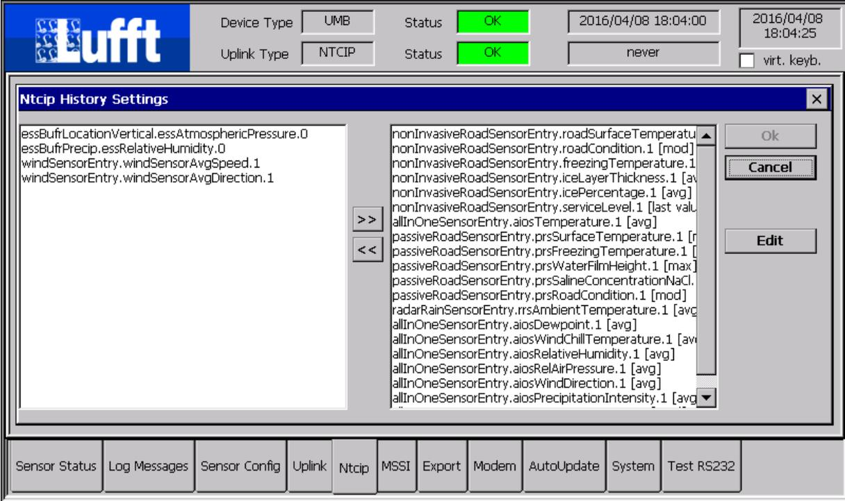
For each OID that is configured for data storage, a “statistics type” can be configured. This statistics type is used to calculate an aggregated value for the reporting interval when retrieving data from the data store, if the reporting interval is greater than the actual store interval (which is fixed to 1 minute).
