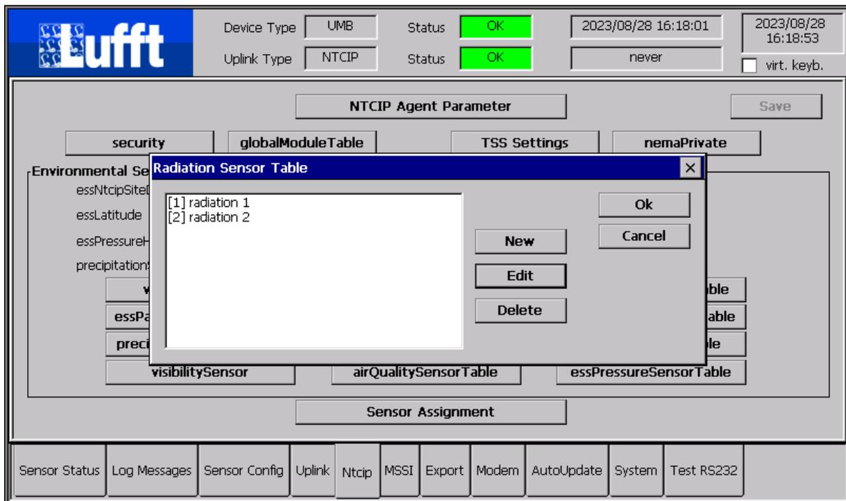
The meta data for each radiation sensor (location information etc.) and thereby the number of sensors in the corresponding table is configured here.
