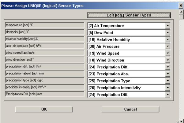
Then a dialog to assign the station sensors to the template job is shown:
