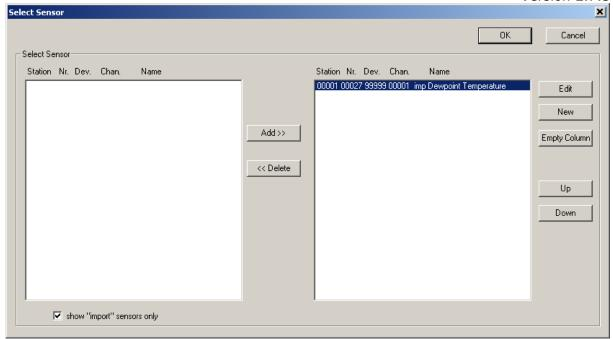
If a station is configured for the export job, only sensors of that station are displayed to be selected. If **show "import" sensors only** is checked (which is the default), only "import" sensors (that have been created using "New") are displayed for selection.
