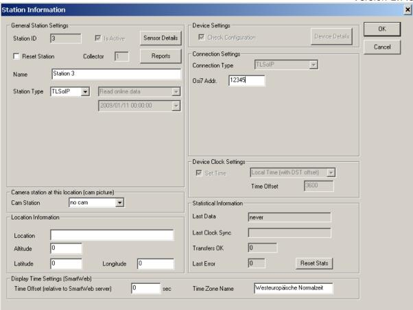
Configuration parameters for a TLSoIP station are (besides general items like an assigned CAM station or the location information) limited to the station name and OSI7 Address.
