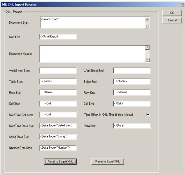
This dialog allows to configure the XML output format for XML Export. The exported XML document always has the following structure:
