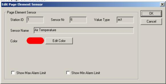
For a line diagram sensor the color of the curve in the line diagram can be specified.
