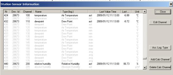
Disabled sensor channels are displayed in gray. For all active sensor channels, the last value time, last value and unit are displayed.
