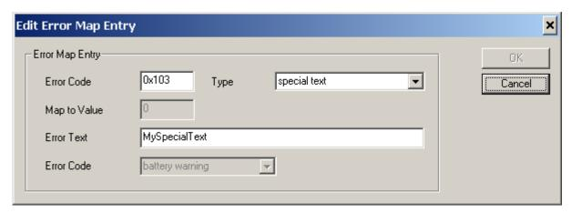
There can only be one entry configured for each error code. The error code 0x0 is used to specify an entry that is valid for all error codes. When processing a measure value with an error code, the list is first searched for an entry with the specific error code of the measure value. Only if no entry with this
