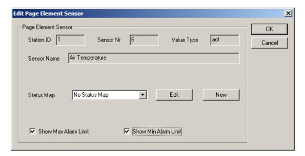
For a "horizontal bar diagram", "color code", "table" or "pictogram", "status mapping" is used to specify which color/text/pictogram is assigned to a specific sensor value.
