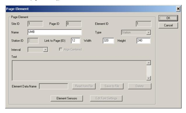
Width and height of the "Station" element specify width and height of the cam picture display for this station on the group status page.
