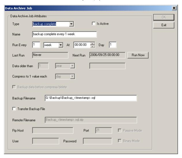
• **Type:** can be "delete", "delete pictures", "compress", "backup" or "backup complete": **delete**: delete measurement data older than the configured time. The deleted data can be backed up automatically before it is deleted.
