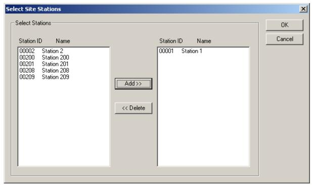
This dialog is used to select the stations to be used on a site. To select a station, mark it in the left list box and click "add". To remove a station mark it on the right list box and click "delete".
