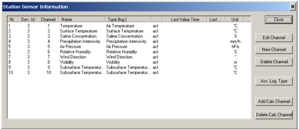
To add a new sensor to a TLSoIP station, you need to enter the FG, Type and Channel for the sensor:
