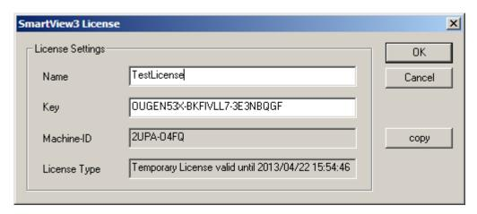
The license is bound to the PC hardware (identified by the specific Machine ID).
