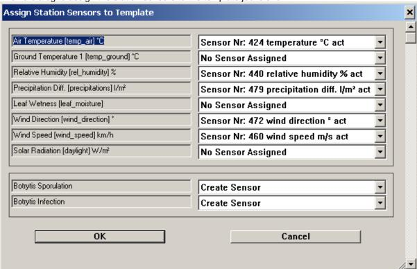
If (which usually is the case) there are no appropriate import sensors for the station available, the sensors will be created. For the pre-defined job templates (the plant disease models), this will be done completely automatically.
