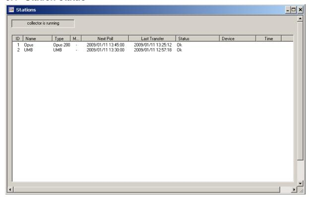
The window shows all configured stations, and the status of the station in Collector, e.g. the status of a station if it is currently polled by collector (and the collector is running).
