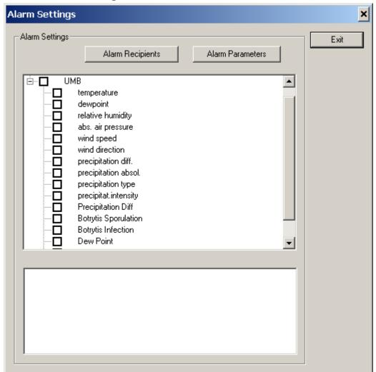
Here you can activate/deactivate alarms for stations and sensors of a station, and for export jobs, by clicking in the appropriate check box.
