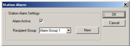
You can select the alarm recipient group for alarms for this station from the box, or create a new group. A "station alarm" is generated if a station could not be polled for new data, or if the station reported an error for a specific sensor (if alarms for that sensor are active as well).
