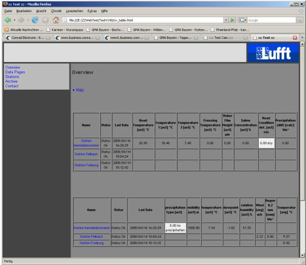
The "table overview" shows status of all stations, and the sensors configured for each station in a table. Sensors with identical logical sensor type, value type and unit are shown in the same column. There is a parameter for the "Overview page" (see below) to configure the maximum number of sensors displayed in one table.
