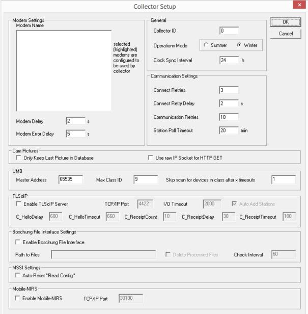
Here you need to select the modem(s) you would like to use with Collector to connect to the stations (if you use dial up connections to your stations). You can assign the modems to different "modem pools".
