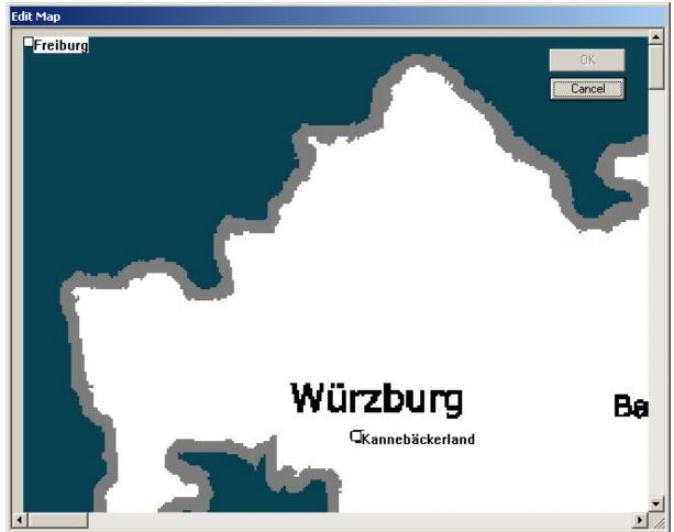
This is the map editor window (Map page only). Click on the white square of the station and move it (by holding the left mouse button) to the desired position on the map, and release the mouse button. If the map is bigger than your screen, you may need to move the station icon, and scroll the dialog, and then move the station icon further.
