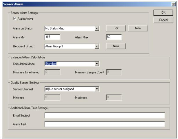
Here you can set/edit the "status mapping" to be used to determine a warning/alarm condition or you can set the lower and upper alarm limits for the sensor. Default is the minimum/maximum value the sensor channel supports.
