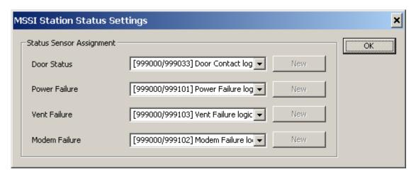
After a sensor channel has been assigned (which creates an appropriate sensor channel for the station), the sensor channel appears in the stations sensor list and can be configured like any other sensor channel of the station.
