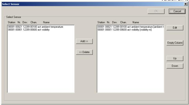
If a station was configured for the export job, only sensors from that station are available on the left side to be selected for the export. A sensor may be selected multiple times. Empty columns can be inserted into the export by clicking "empty column" on the right side.
