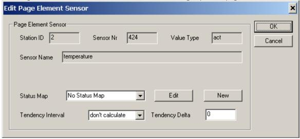
Status-Map: the status mapping to be used to display text/color mapping for a sensor value in the table (see status mapping).
