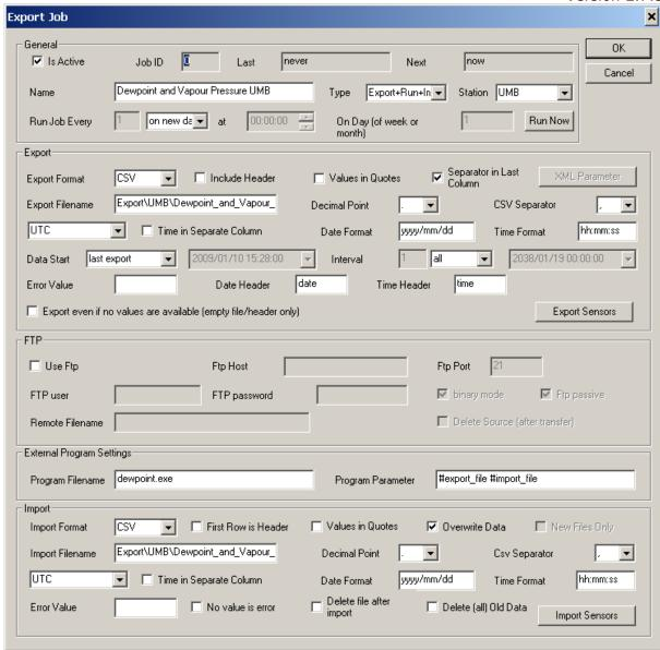
Following parameter must be set for the dew point calculation:
