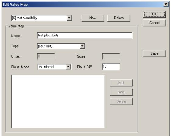
To check if the current value is a valid value, the last values for this sensor (within the last 24 hours) are read from the database. If there is no valid value for the sensor within the last 24 hours, no plausibility checking is applied.
