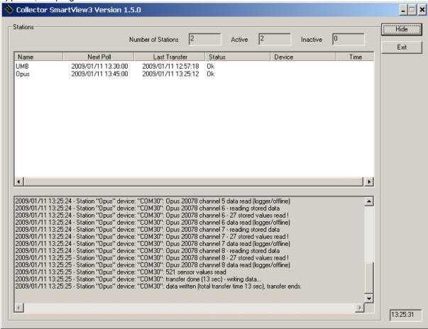
The configured stations are shown in the upper part of the window, showing the next station due to be polled first.
