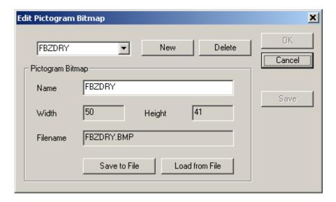
Pictogram bitmaps can be loaded from a file on the hard disc, or written to a file on the hard disc. The name for the pictogram bitmap can be edited.
