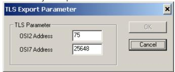
Note: the file that is created by this type of export contains one TLS TC57 (Inselbus) data telegram with "result values" (measure values) for function group (FG) 3 sensors for one timestamp. TLS sensor type and channel assignments are part of the export sensor settings (see below). The values need to be scaled or converted to the appropriate TLS data types or coding as appropriate.
