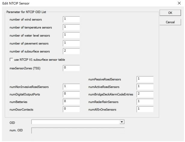
The parameters determine which entries are available in the OID combo box. If the station Meta data has been read from the station, the number of sensor entries for each table is set by the stations actual configuration.
