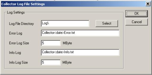
The default filenames for error and info log file are "CollectorError.txt" and "CollectorInfo.txt" respectively. If you want to keep log files for Collector on a daily basis, please add the <date> tag to the filenames as shown above.
