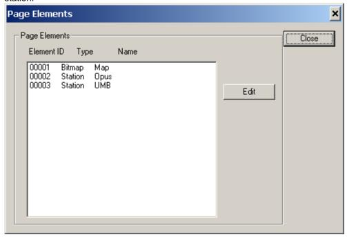
The sensors assigned to the "station" element determine, which sensor values are displayed when you "scroll over" the station icon with the mouse (map display). They determine which sensors (and in which order) are shown on the overview table as well.
