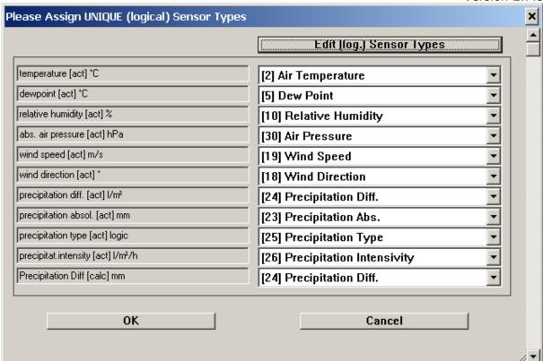
You can select a logical sensor type from the drop down box. If there is no pre-defined sensor type that fits you sensor, you can create a new sensor type using the button "Edit (log.) Sensor Types.
