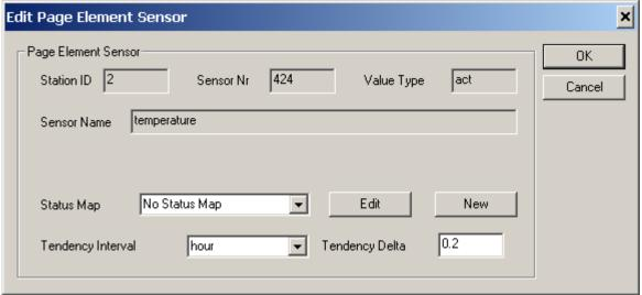
The tendency is always calculated by comparing the current sensor value with the value before. The Tendency Interval specifies the maximum time period an older value may actually be older – if there is no value within that time period, no tendency is calculated.
