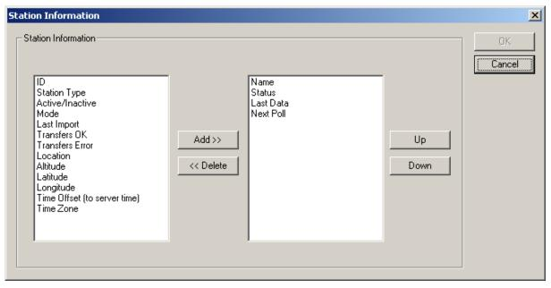
Select which station information is included in the station information table on the station page. For NTCIP stations, the additional elements "NTCIP station meta data" and "NTCIP module table" can be selected.
