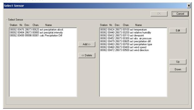
This dialog shows sensors to be selected. This dialog is used wherever Sensors can be selected within SmartView3 (e.g. Sensors for a data page, sensors for diagrams or tables, sensors to be exported etc.).
