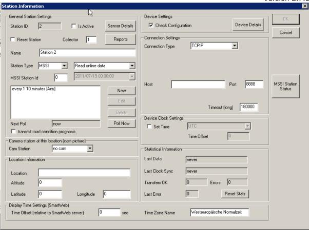
For MSSI stations, the additional option "transmit road condition prognosis" is available. Note that this is a non-standard extension to the MSSI protocol, and might not be supported by the station. Please only activate this option if the station supports the road condition prognosis extension (e.g. Lufft LCom Version 1.7.0 or higher).
