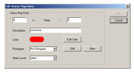
For "Pictogram" displays a bitmap must be assigned to all entries of a "Status Map".
