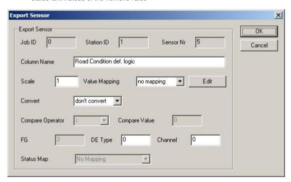
Note for export format "TLS trace file": the sensor values need to be scaled to the appropriate TLS data formats/units (e.g. temperatures in TLS are in 1/10 °C, so they need to be scaled by 10, water film in TLS is in 1/100 mm so they need to be scaled by 0.1 if the "source sensor" is in  $\mu$ m) or converted (e.g. road condition coded in "Lufft def" need to be converted to TLS DE Type 70 coding using an appropriate value mapping).
