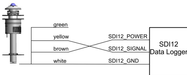
Figure. 1: Connecting to a logger with integrated power supply
