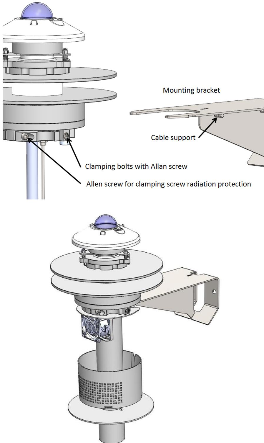
Fig. installation, WS3000
