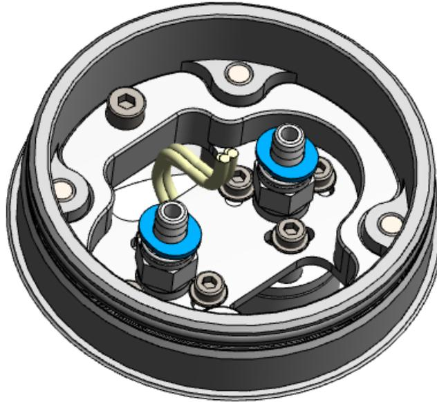
Fig: Pressure sensor connections
