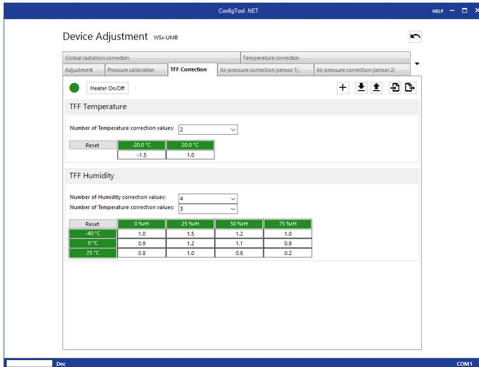
Please note that the grid points can only be defined in an ascending order. When entering data into the table this is automatically checked, and any deviations are marked in red.
