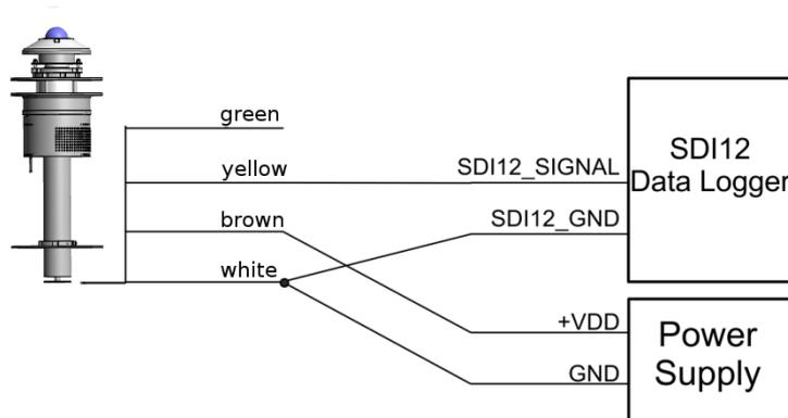
Figure. 2: Connecting to a logger and a separate power supply
