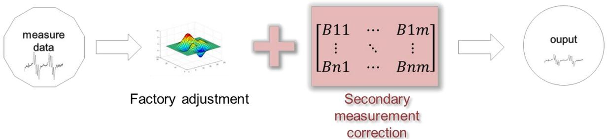
The customized correction function is based on an interpolation matrix which can consist of up to ten grid points with their related correction values. An indication of one grid point only equals a simple offset correction. If a second grid point is included, this equals a correction consisting of offset and gradient.
