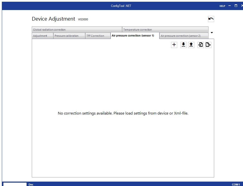
When the adjustment dialogue is accessed for the first time there is no adjustment set available. A new set can be created offline, so that a correction can be generated without a sensor connected. In the upper right corner there are icons for loading, saving and transmitting the correction functions:
