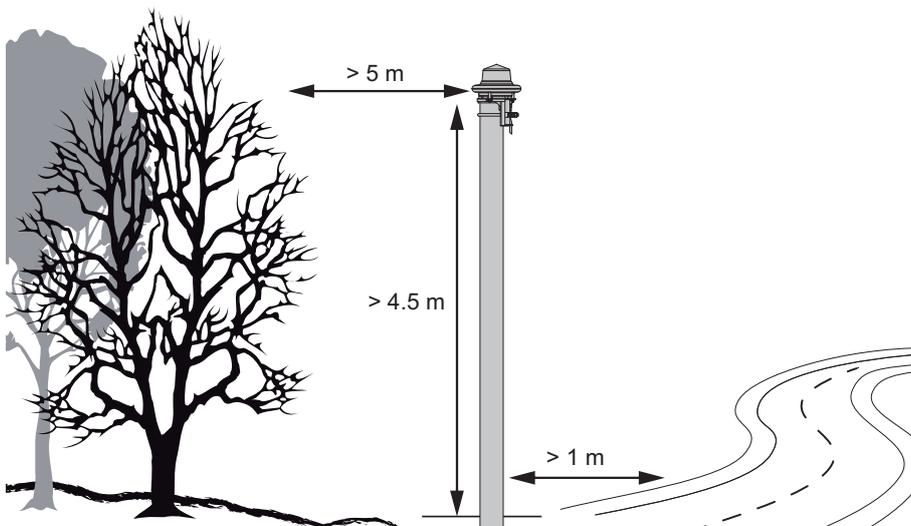
If the device is used to observe the weather for road and traffic control systems, carry out the following installation steps:
