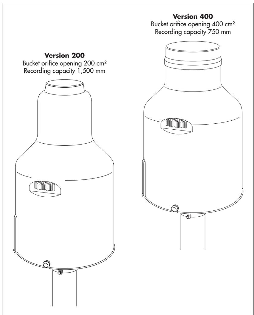
Every 6 seconds, the precipitation gauge determines the weight of the collecting bucket including its content using a resolution of 0.001 mm (= raw data). The difference between this measured value and the basic weight of the empty collecting bucket gives the current bucket content.
