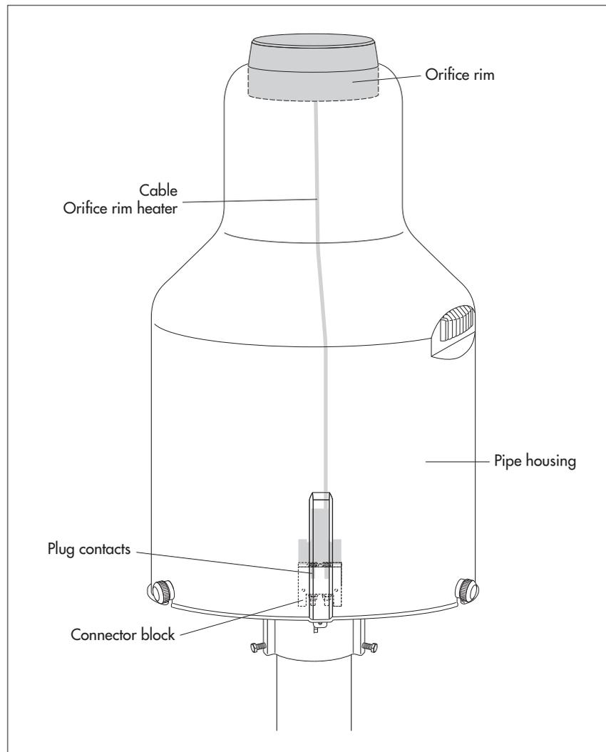
The OTT Pluvio<sup>2</sup> L unit heats the orifice rim until the target temperature of +4 °C (factory setting) is reached – as far as heating power and ambient conditions allow. To achieve this, the heater control system measures both ambient and orifice rim temperatures and uses these values together with the target temperature to calculate the pulse/pause ratio. Depending on this value, the heater control system supplies electricity to the heating element for 5 to 120 seconds.
