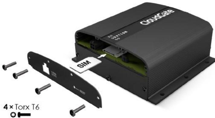
A Torx screwdriver T6 is needed to open the side cover! After the procedure please close the Cloud Gate central unit box.
