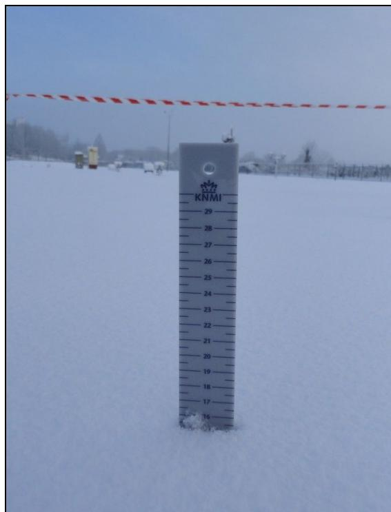
**Figure 5. The graduated snow ruler used by the voluntary precipitation observers in the Netherlands. The range of the ruler is 0-30 cm with a resolution of 0.5 cm.**
