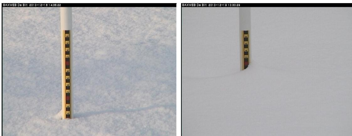
**Figure 12. Camera images of snow ruler SR2 on 18 December 13:35 (left) and 19 December 09:30 UTC (right). Note the pile-up of snow along the ruler, discussed in the text, in the right-hand image.**
