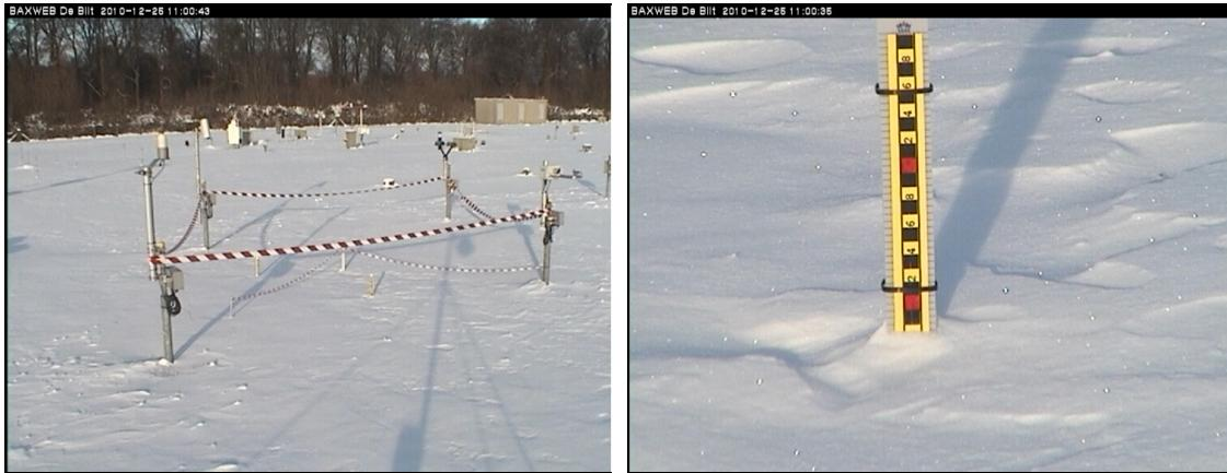
**Figure 4. Camera images of the snow depth testing area (left) and snow ruler SR2 (right) on 25 December at 10:00 UTC.**
