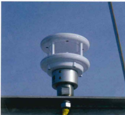
Lufft V200A ultrasonic wind sensor on Dongfang wind turbine in China
