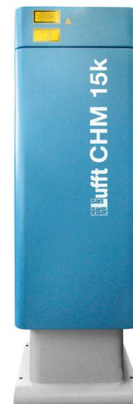
The highly accurate and stable Lufft CHM 15k cloud height sensor features high optical sensitivity for accurate results and a great measuring range of up to 15km. It's eye-save laser is protected by a double case housing and works in foggy, rainy, icy and hot weather conditions.
