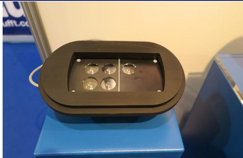
**The Lufft cloud simulator enables the user to quality check the ceilometer CHM 8k in lab and in the field.**
