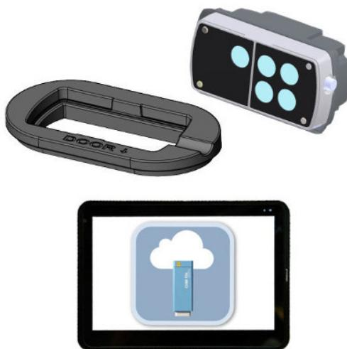
**The Lufft CHM Simulator simulates the cloud height for the ceilometer CHM 15k in order to check its measurement accuracy.**
