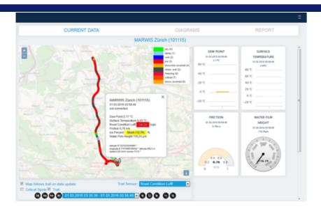
ViewMondo, the flexible Lufft Road & Runway Management Software, that collects different types of data, checks the data for plausibility and evaluates data and recommendation out of the data in according to your needs!
