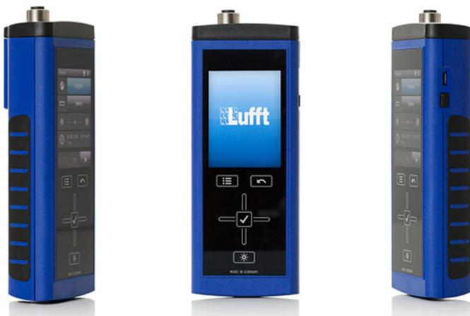
**The most precise and flexible all-rounder instrument for professional applications-easy to handle and robust for measurement of Temperature/Humidity, flow, co2 and air pressure**
