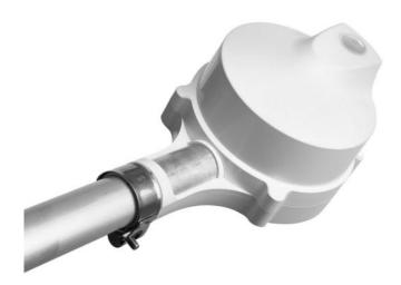
All-in-one weather sensor with measurement of temperature, relative humidity, air pressure, wind velocity / direction, precipitation amount / intensity / type, UV index, sun direction, brightness and twilight and global radiation
