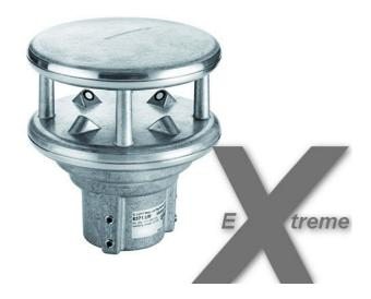
**VENTUS-X: Additional transducer heater for most eXtreme** environmental conditions! Extremely precise and maintenance-free measurement of wind speed and wind direction even in the lowest temperature
